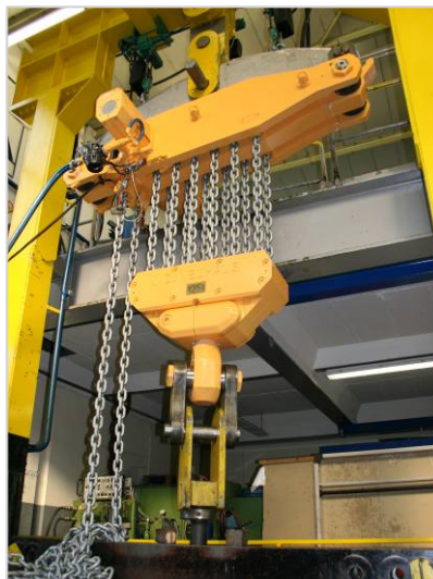
Fig. left: EH 125 Lifting Unit in test stand
