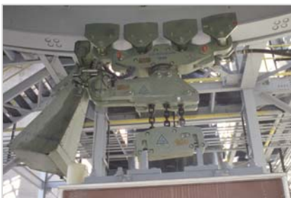
The EH 80 Monorail Hoist, able to negotiate curves, shown in a typical cement industry environment.
